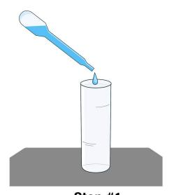
**Step #1** Using the Pipette, Add Seven (7) drops of drinking water into the Test Vial.
