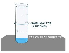
**Step #2** Swirl Test Vial for 10 seconds. Make sure all liquid is at the bottom of the Test Vial by tapping it gently on a flat surface.
